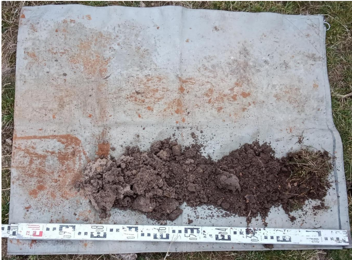
Figure 22: Soil profile – Lot C effluent dispersal area.
