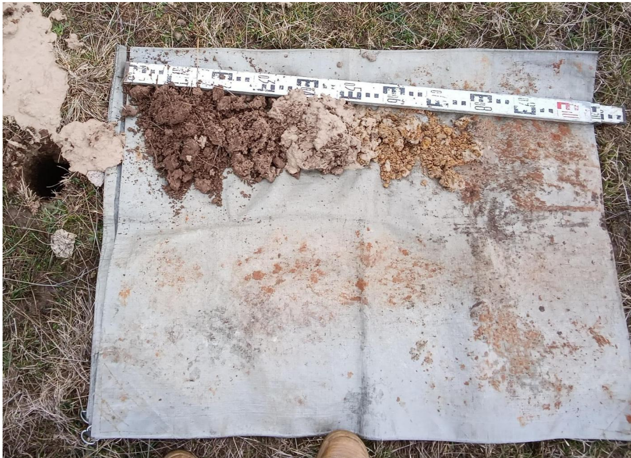
Figure 21: Soil profile – Lot B effluent dispersal area.
